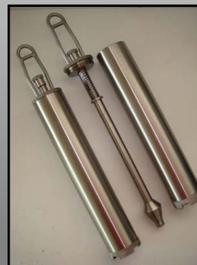
Bottom sampler for liquid tanks
