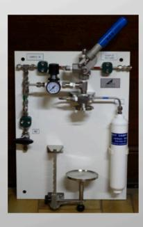
Closed loop process liquid samplers, with or without N2 purge system for cleaning purposes. N2 pressure max. 6 bar and pressure controlled to clean the injection needles. Systems are wall mounted, all wetted parts in stainless steel.
